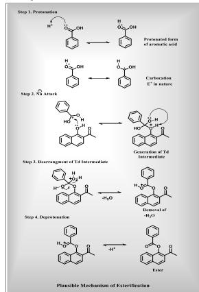
**Fig. 2.** Plausible mechanism of esterification of aromatic acids.
