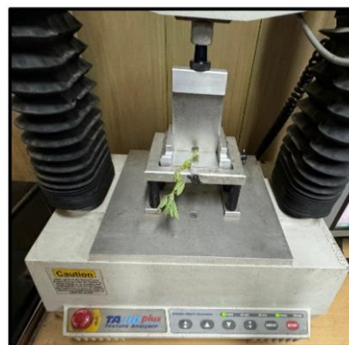
Fig. 3. Measurement of cutting fore of fenugreek by texture analyzer.
