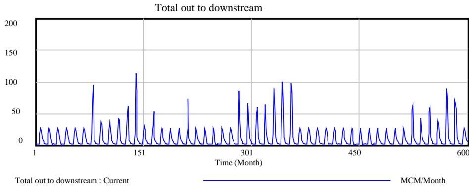
Fig. 18. Input discharge entering the Urmia Lake after Shahrchay Dam construction.
