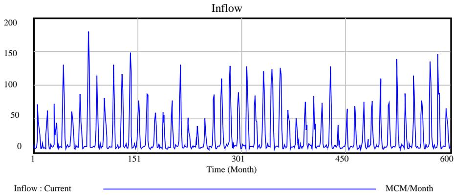
**Fig. 15.** Input discharge entering the Urmia Lake before Mahabad Dam construction.
