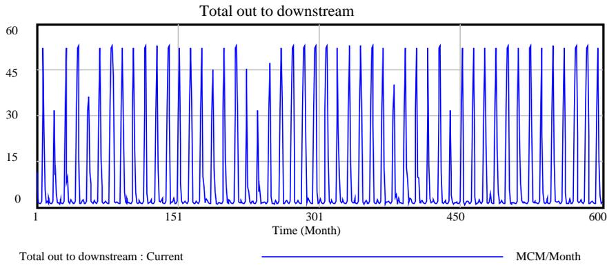
**Fig. 12.** Input discharge entering the Urmia Lake after Zarrinerud Dam construction.
