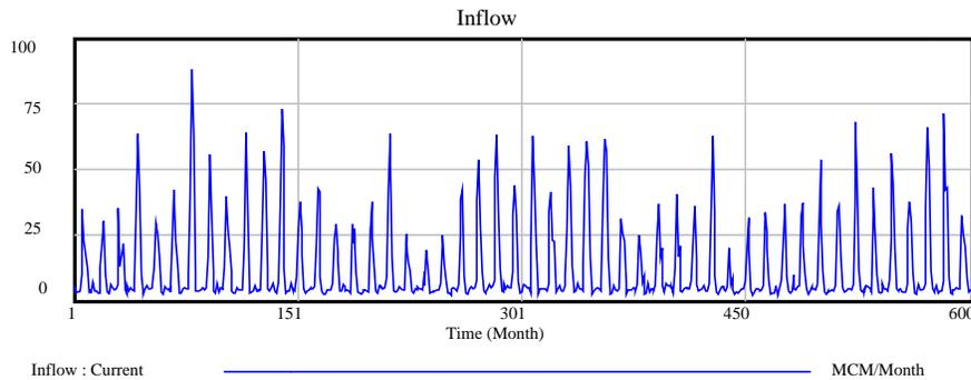
**Fig. 7.** Input discharge entering the Urmia Lake before Alavian Dam construction
