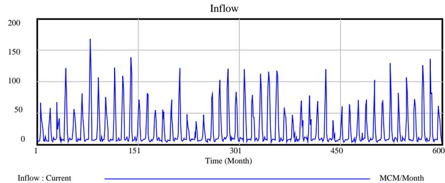
**Fig. 17.** Input discharge entering the Urmia Lake before Shahrchay Dam construction.
