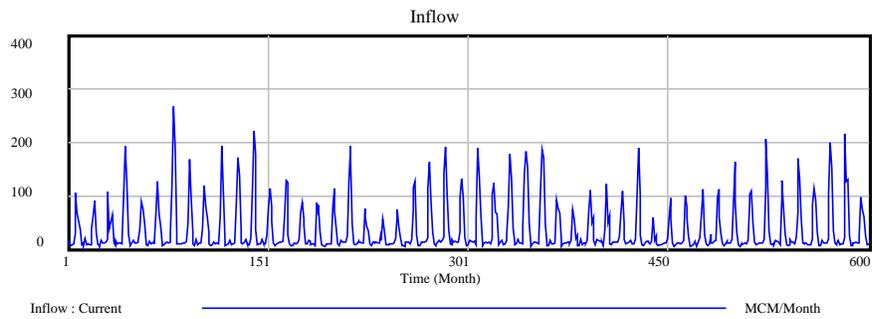
**Fig. 11.** Input discharge entering the Urmia Lake before Zarrinerud Dam construction.
