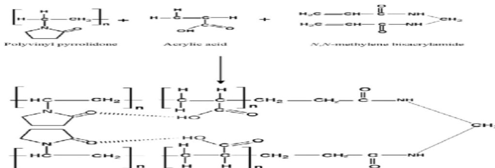
**Fig. 1.** Possible structure of polyvinylpyrrolidone/acrylic acid hydrogel.
