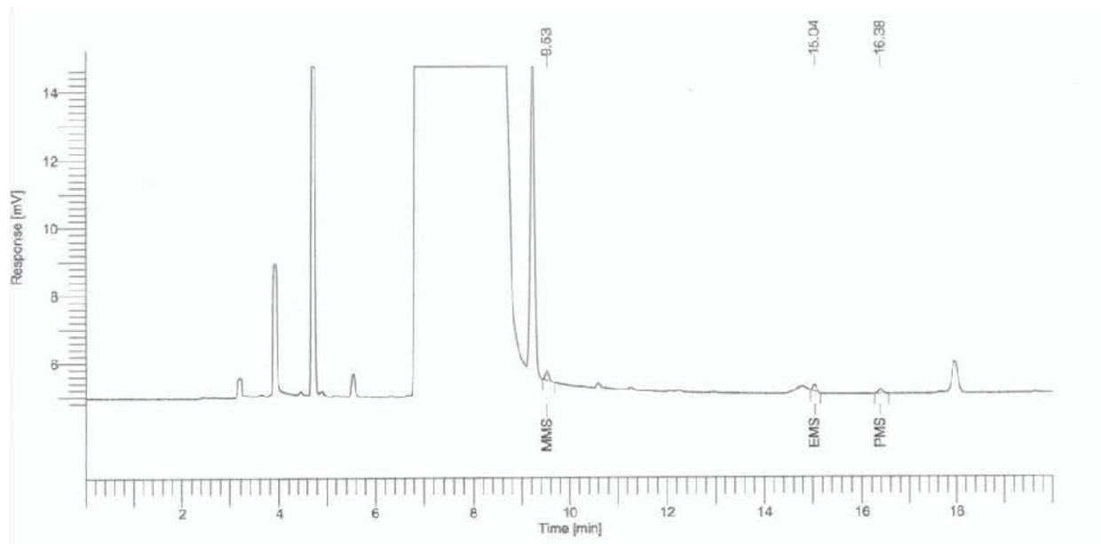
**Fig. 2.** Gas chromatogram for MMS, EMS and IPMS.
