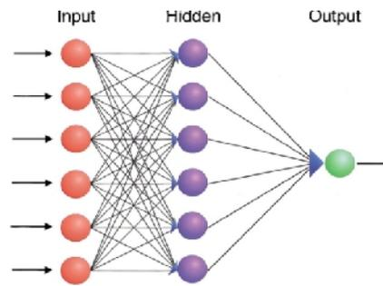
Fig. 1. The structure of a perceptron with one hidden layer.
