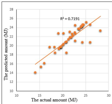
Fig. 5. The relationship between predicted using neural networks and actual of energy output (milk).
