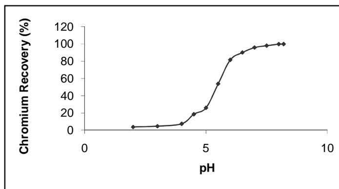
**Fig. 1.** Effect of pH on Chromium recovery from waste water.
