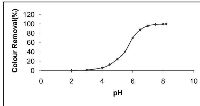
Fig. 2. Effect of pH on colour removal from waste water.
