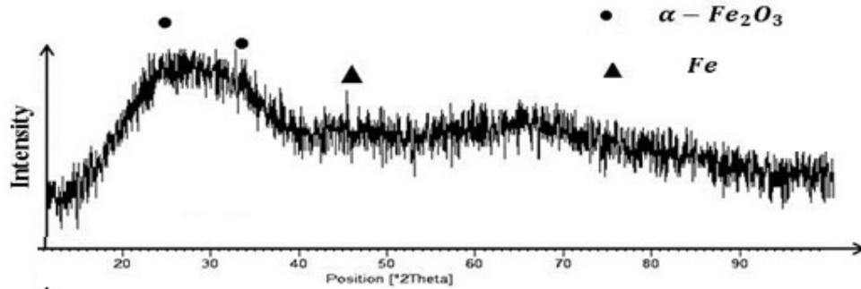
Fig. 1. XRD pattern of Ferric Nanoparticles deposited by CBD method.
