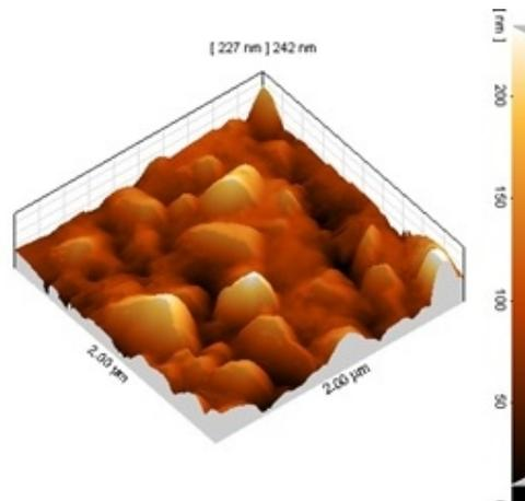
Fig. 3. The AFM graph of Ferric Nanoparticles deposited by CBD method.
