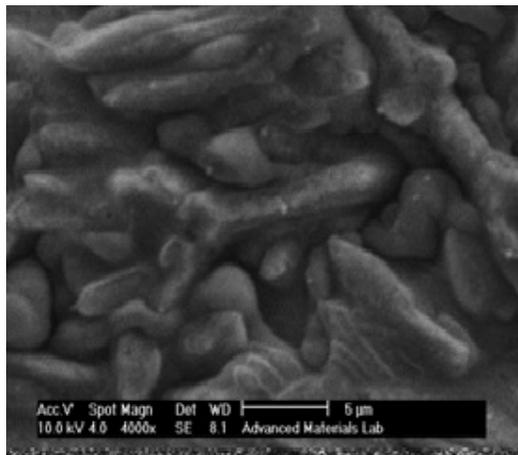
Fig. 2. The SEM image of Ferric Nanoparticles deposited by CBD method.
