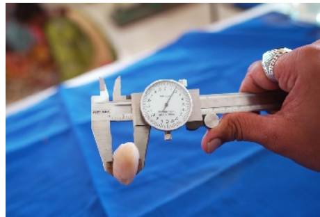
Plate 2: Measurement of length and width of water chestnut kernels.
