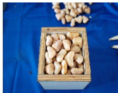
Plate 3: Measurement of bulk density of whole water chestnut and kernels.
