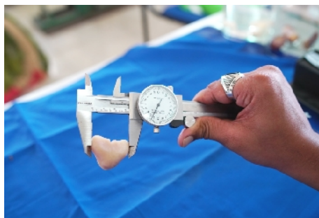
Plate 2: Measurement of length and width of water chestnut kernels.
