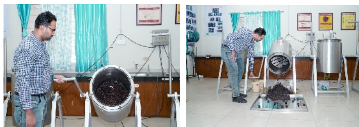
Plate 6: Unloading cooked water chestnut by tilting the pressure vessel.
