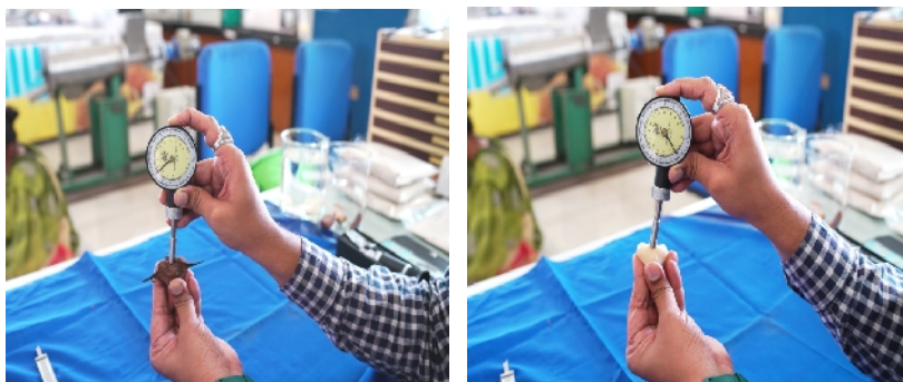
Plate 4: Hardness measurement of whole water chestnut and kernels.
