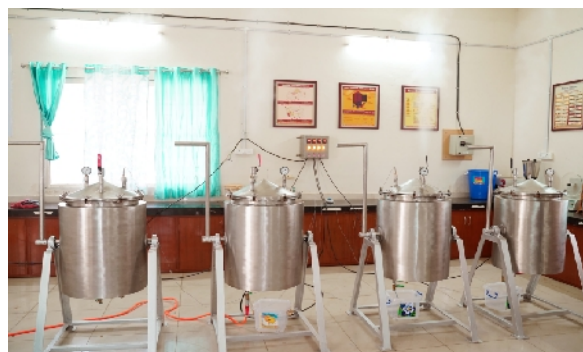
Plate 5: Pressure vessels assembly with RTD controller.
