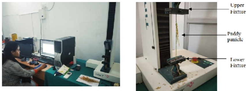
Fig. 2. Measurement of detachment force of grain by Universal Testing Machine.
