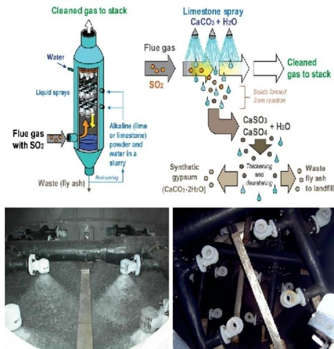
**Fig. 3.** FGD Gypsum production in thermal power plants.
