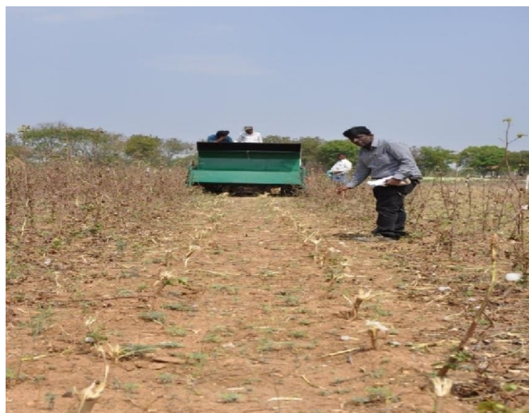
Plate 1. Field evaluation of cotton stalk harvesting machine.
