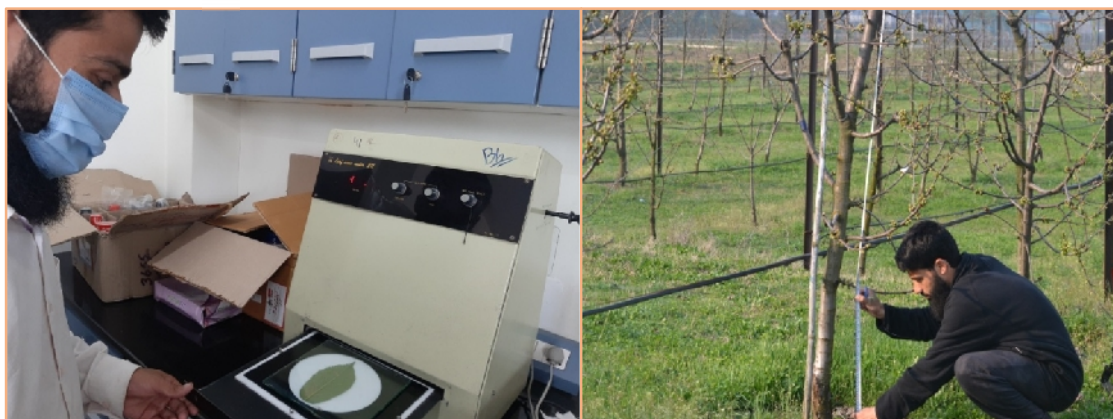
Fig. 2. Leaf area and tree height measurement using Systronics leaf area meter-211 (left) and measuring staff (right), respectively.
