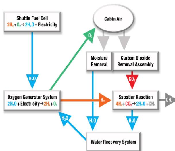
Fig. 3. NASA and ISS station model for produce essential material for astronauts (www.nasa.com).
