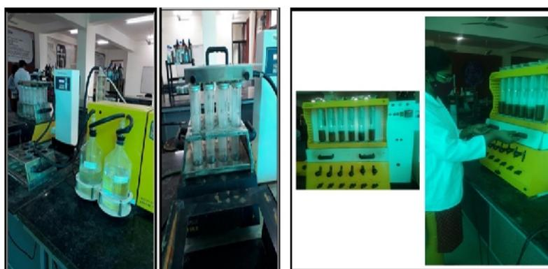
**Fig. 1. A.** Estimation of Nitrogen by Kjeldhal apparatus; **B.** Estimation of crude fibre by KEL Plus.
