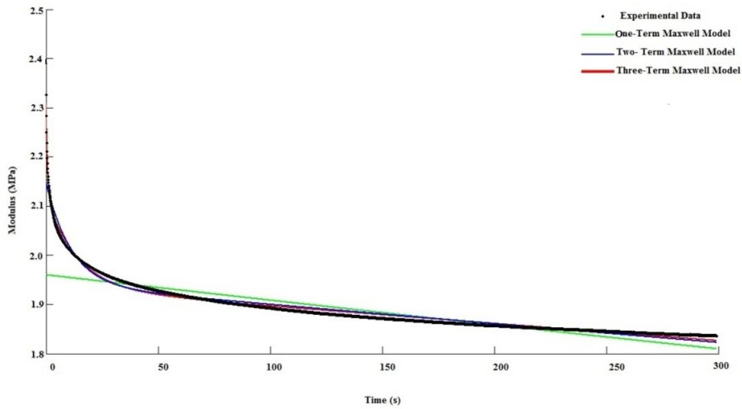
Fig. 9. Roasted chickpea stress relaxation behavior by fitting one, two and three term Maxwell models to experimental data.
