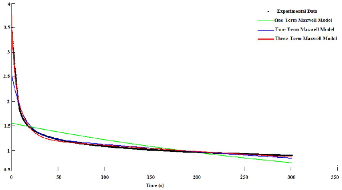
Fig. 8. MT stress relaxation behavior by fitting one, two and three term Maxwell models to experimental data.
