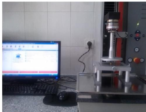
**Fig. 3.** Chickpea's conditions for Stress relaxation test.
