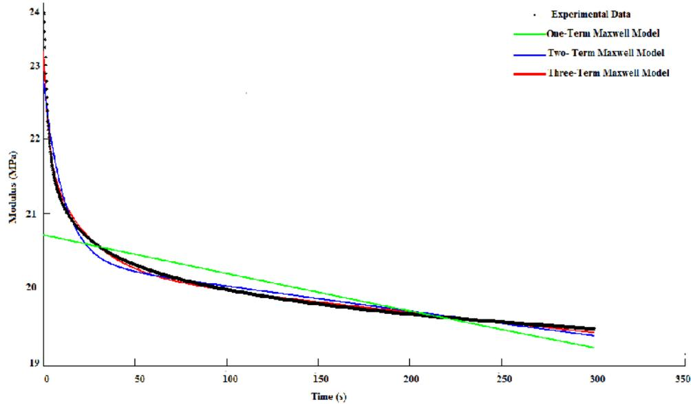
Fig. 6. FHT stress relaxation behavior by fitting one, two and three term Maxwell models to experimental data.
