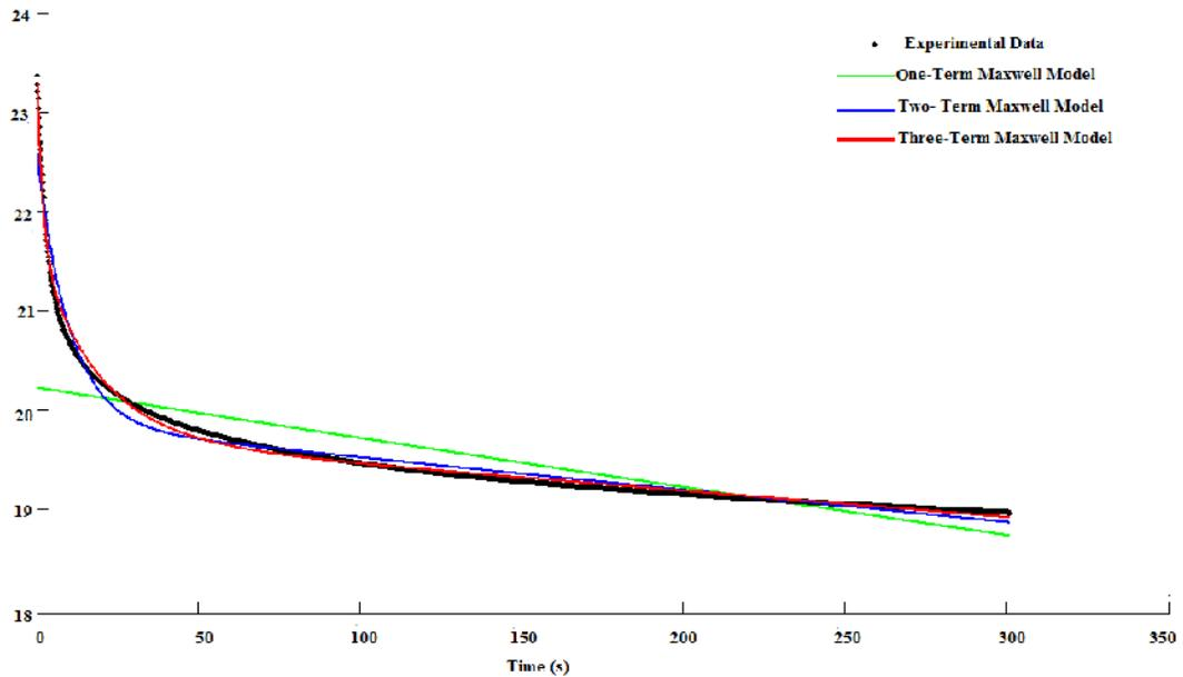
Fig. 7. SHT stress relaxation behavior by fitting one, two and three term Maxwell models to experimental data.
