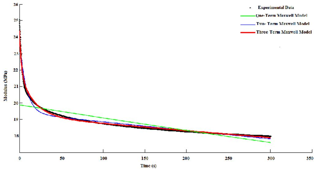
Fig. 5. Row Chickpea stress relaxation behavior by fitting one, two and three term Maxwell models to experimental data.
