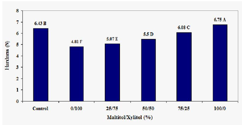
**Fig. 6.** Effect of sugar substitutes concentration on hardness of chocolate.
