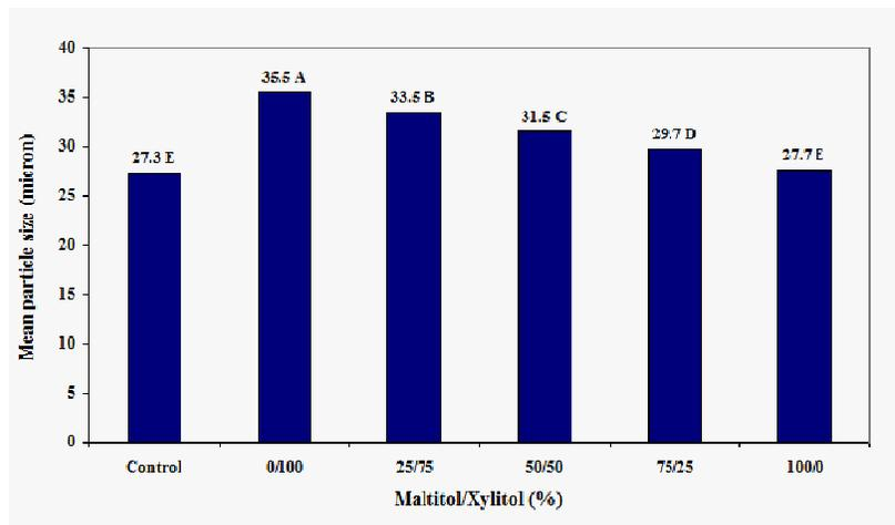
Fig. 2. Effect of sugar substitutes concentration on mean particle size of chocolate.
