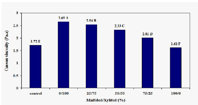
Fig. 3. Effect of sugar substitutes concentration on Casson viscosity of chocolate.
