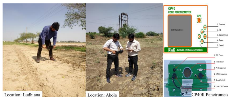
Fig. 2. Measurement of cone index at different locations of India by hand operated penetrometer.
