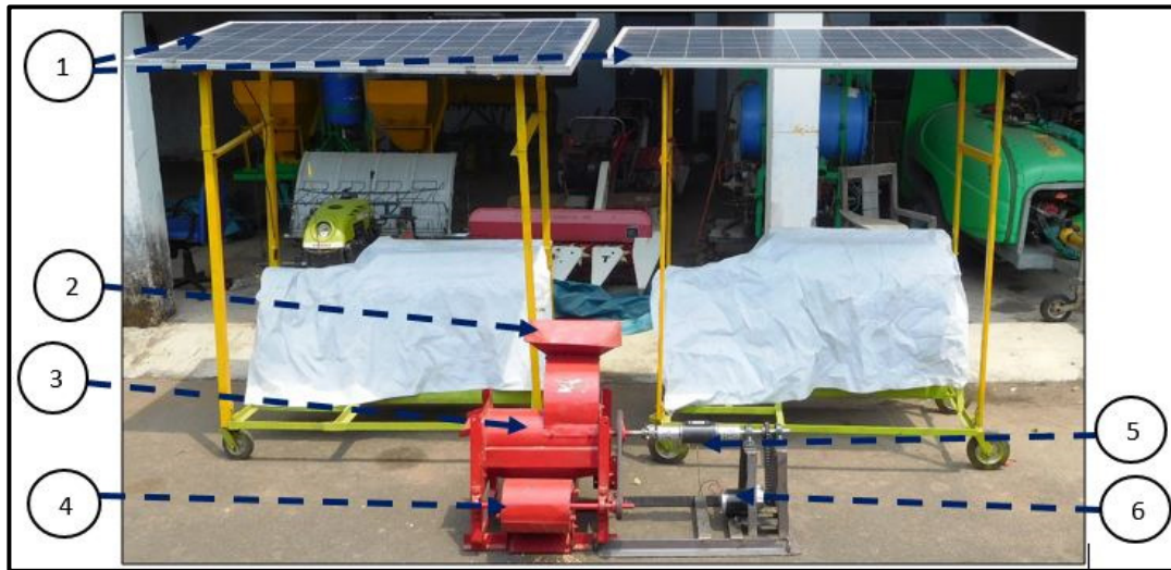
1. Solar panel 2. Feeding chute 3. Threshing cylinder 4. Blower 5. Torque transducer 6. DC motor
