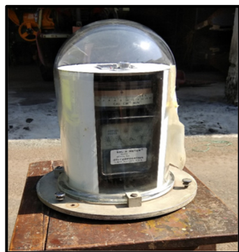
Fig. 6. Measurement of solar radiation by a pyranometer.
