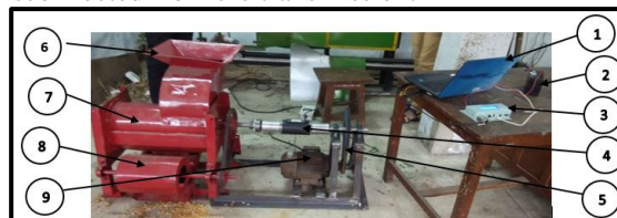
1. Laptop; 2. Battery; 3. DUT; 4. Torque transducer; 5. Belt and pulley transmission system; 6. Feeding chute; 7. Cylinder; 8. Blower; 9. AC motor
