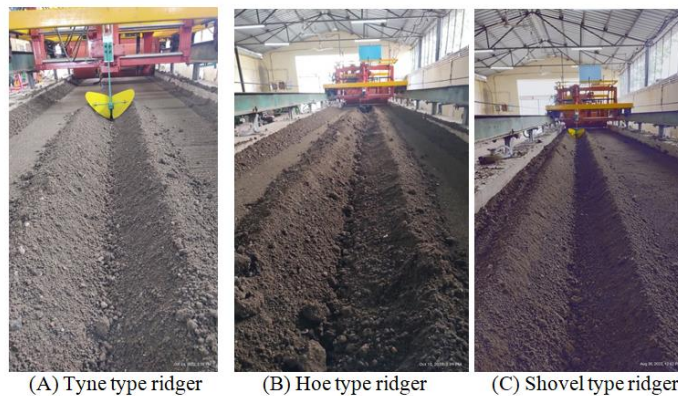
Plate 2: Testing of the ridgers at maximum working depth and width of cut
