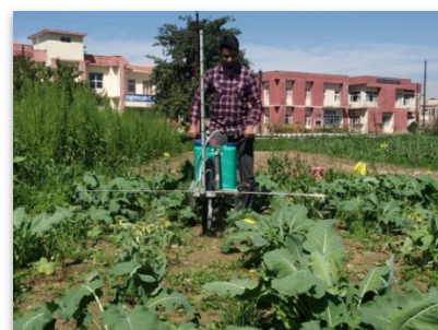
Fig. 1. Evaluation of the developed wheel operated boom sprayer in field of knoll khol crop.
