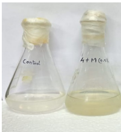
Fig. 5. After 7 Days of Incubation Cronobacter sakazakii Degrading MCP (1000ppm) on MSM Media.
