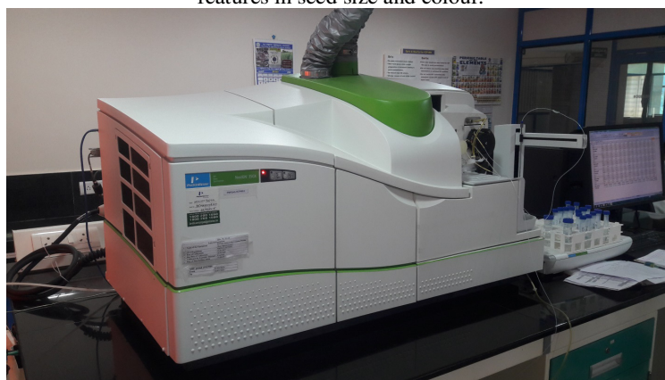
Plate 2. Inductively coupled plasma mass spectrometry (ICP-MS) technique ( Instrument make: Perkin Elmer and Model name: Nexion 350X).
