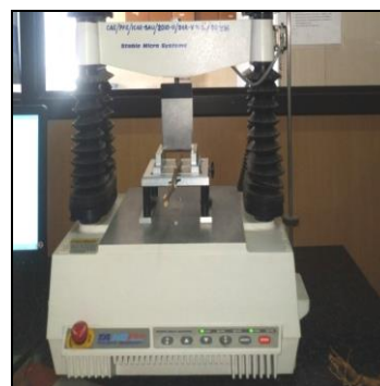
Fig. 3. Measurement of cutting force of cotton stalk.
