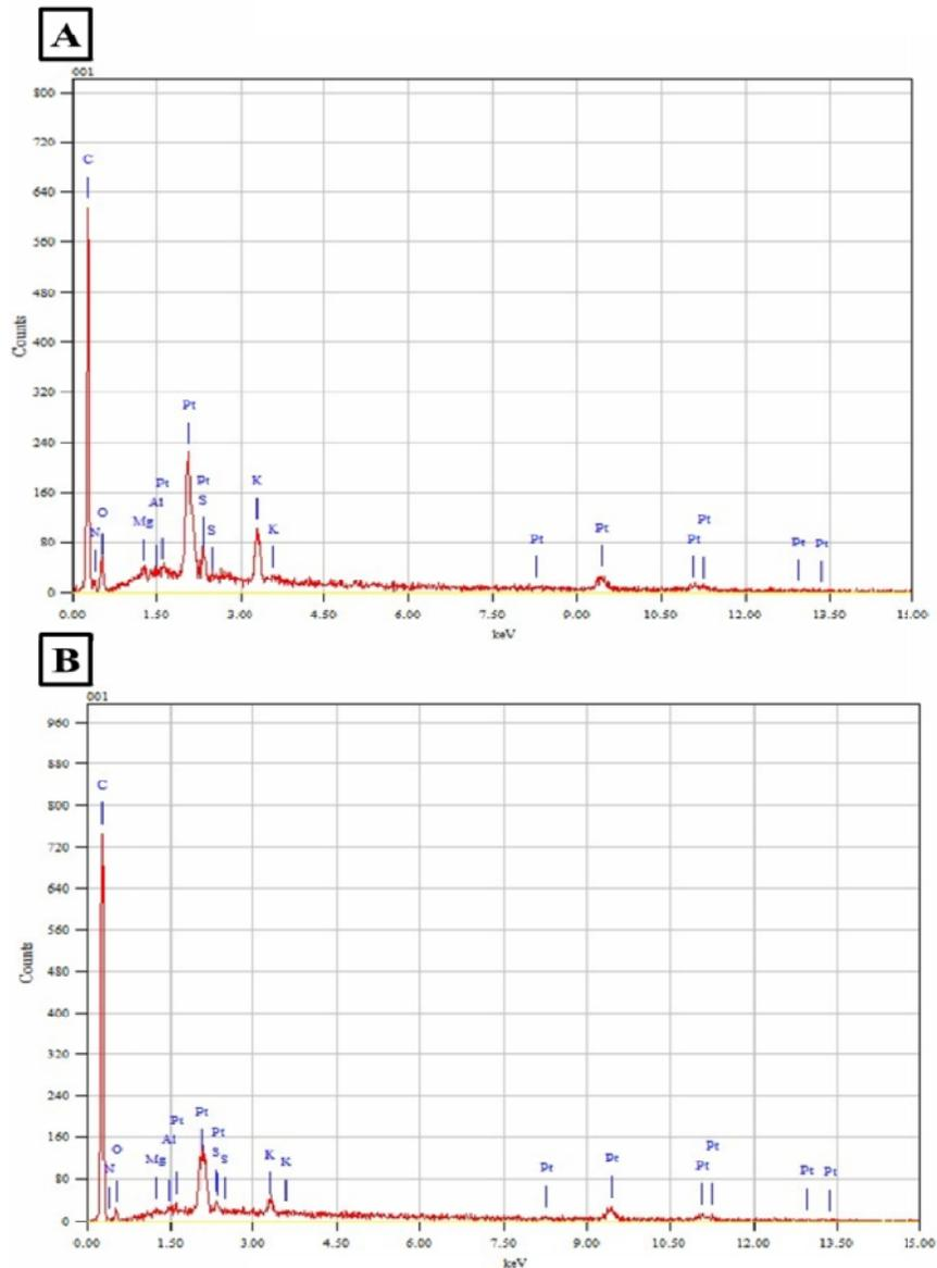
**Fig. 3.** EDX analysis showing the elemental composition of the areas (blue boxes) shown in Figure 2. A) *A. muricarpum*, (B) *E. dalican*.
