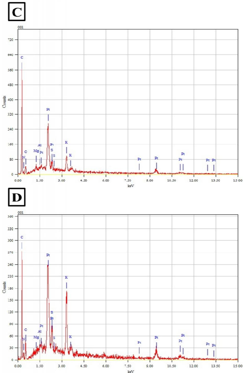
**Fig. 3.** EDX analysis showing the elemental composition of the areas (blue boxes) shown in Figure 2. (C) *E. philippinensis* and (D) *H. conoidea*.
