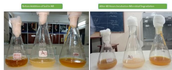
Fig. 6. Microbiological decolorization of textile dyes by action of microorganisms.
