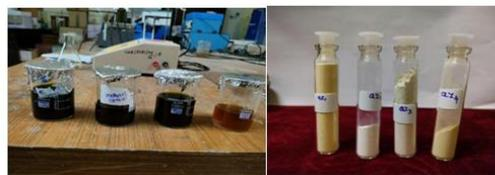
1. Extract in different solvents (Ethanol, Methanol, Acetone and Water); 2. Prepared ZnO Nanopowders in four solvents.
