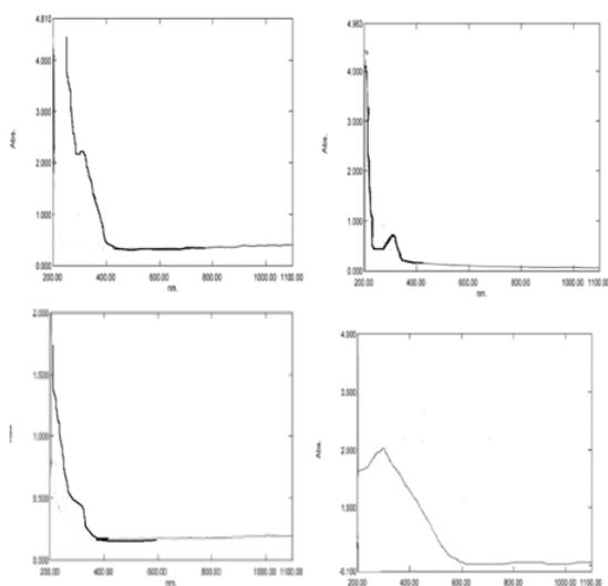
1. UV absorbance of ZnO NPs solvent ethanol; 2. UV absorbance of ZnO NPs solvent acetone; 3. UV absorbance of ZnO NPs solvent methanol; 4. UV absorbance of ZnO NPs solvent water
