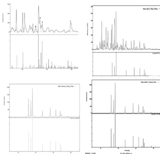
1. XRD ZnO NPs solvent ethanol; 2. XRD ZnO NPs solvent Acetone; 3. XRD ZnO NPs solvent Methanol; 4. XRD ZnO NPs solvent Water.
