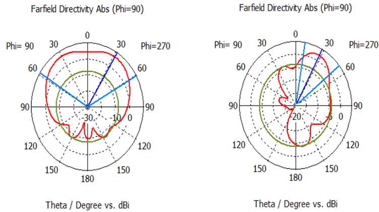
**Fig. 6.** Polar plot of Directivity 90 for phi = 90 for EBG patch antenna.
