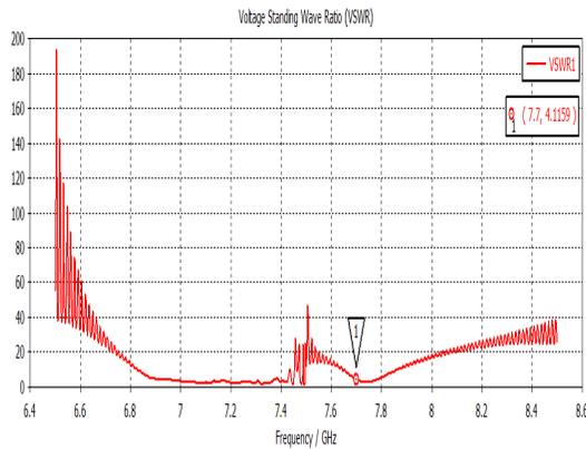
**Fig. 11.** VSWR Curve of EBG Structure of Patch Antenna.
