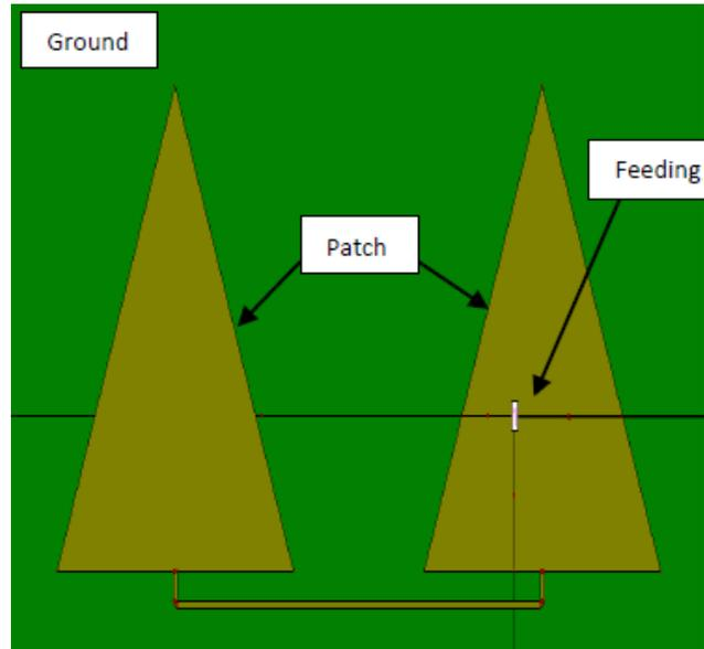
Fig. 2. Patch element antenna array.
