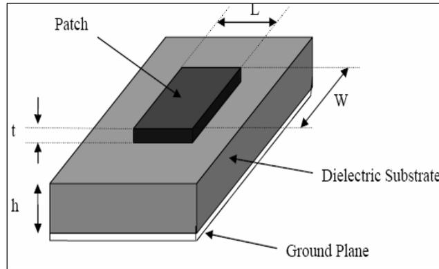
Fig. 4. Microstrip Patch Antenna.
