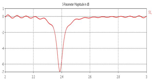
Fig. 1. RL curve of an antenna.
