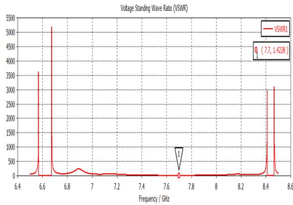
**Fig. 10.** VSWR Curve of Non EBG Structure of Patch Antenna.
