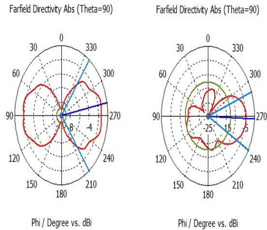
**Fig. 8.** Plot theta = 90 for antenna, directivity for theta = 90 EBG based antenna.
