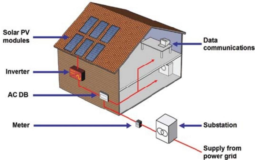
Fig. 3. Grid-connected solar PV system configuration.
