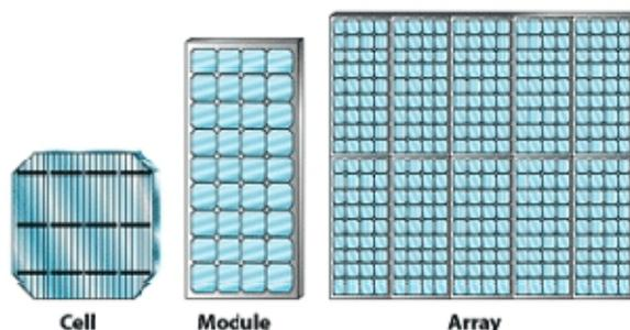
Fig. 6. Cell to module to array.
