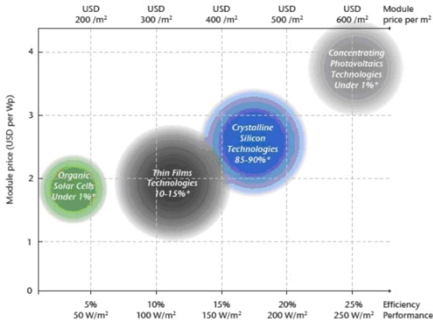
Fig. 5. Performance and price range of different PV technologies.
