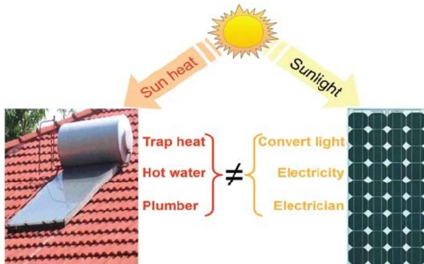
Fig. 1. Conversion of solar heat and light to useful energy.
