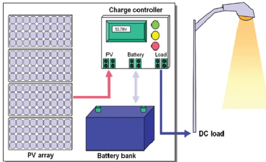
Fig. 4. Off-grid solar PV system configuration.
