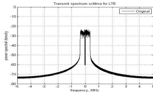
**Fig. 12.** Power spectral density of SC-FDMA.
