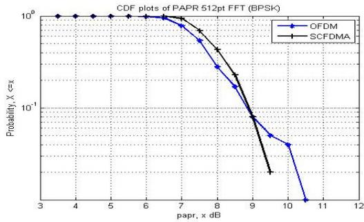
**Fig. 9.** CCDF comparison of PAPR 512pt FFT (BPSK)
