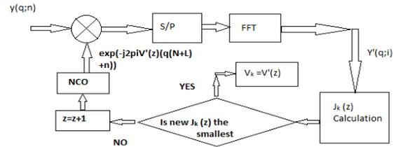
**Fig. 6.** Block diagram of CFO estimation block.
