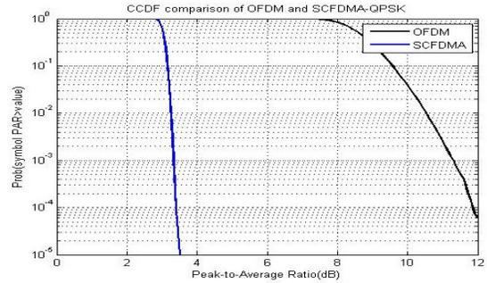
**Fig. 7. CCDF comparison of PAPR 128pt FFT (QPSK).**
