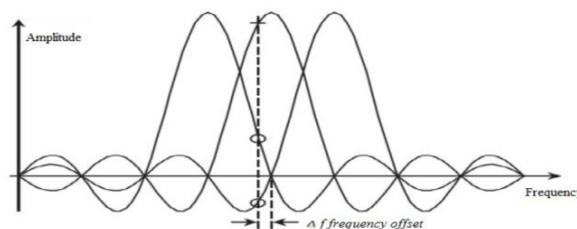
Fig. 4. ICI arises due to frequency offset.
