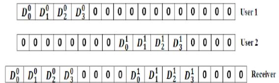
Fig. 2. An exemplary LFDMA subcarrier mapping with sub-bands.
