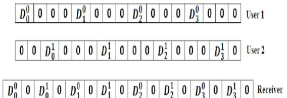
Fig. 3. An exemplary IFDMA subcarrier mapping with sub-bands.
