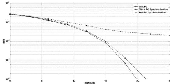
Fig. 13. BER performance of used method.
