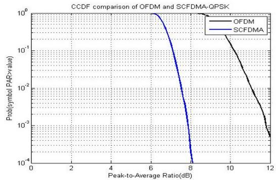
**Fig. 8. CCDF comparison of PAPR 512pt FFT (QPSK).**
