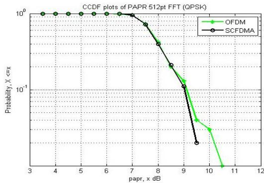
**Fig. 10.** CCDF comparison of PAPR 512pt FFT (QPSK).
