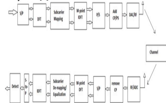
Fig.1. Block diagram of SC-FDMA.
