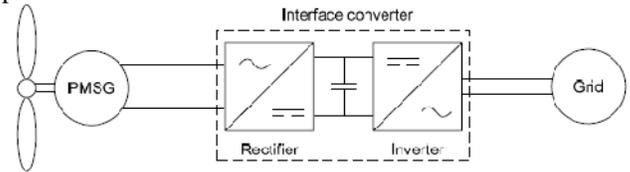
Fig. 5. Block Diagram of WECS.
