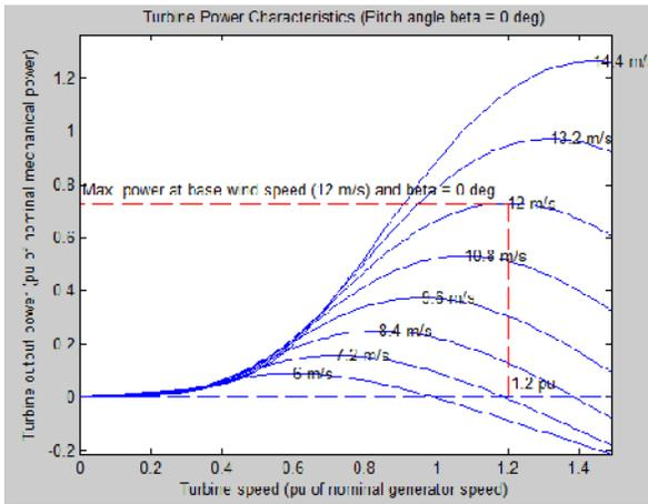
Fig. 7. Wind turbine power characteristics.
