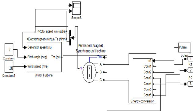
Fig. 6. Simulink Model of WECS.
