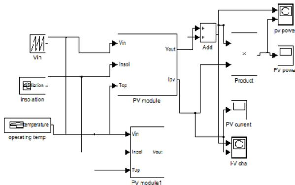
Fig. 2. Simulink model of PV module.
