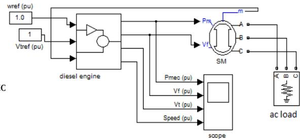
Fig. 8. Simulink diagram of Diesel generator.
