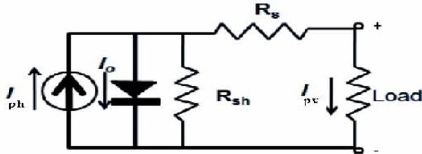
Fig. 1. Equivalent circuit diagram of a solar cell.
