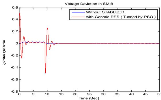
**Fig. 6.** Voltage deviation without PSS & with PSO based PSS fault at  $t = 5$  sec ( $\Delta T = 0.05$ p.u).
