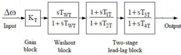
Fig. 1. Structure of Power System Stabilizer.
