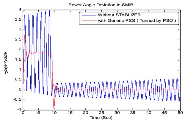
**Fig. 5.** Power Angle without PSS & with PSO based PSS fault at  $t = 5$  sec ( $\Delta T = 0.05p.u.$ ).
