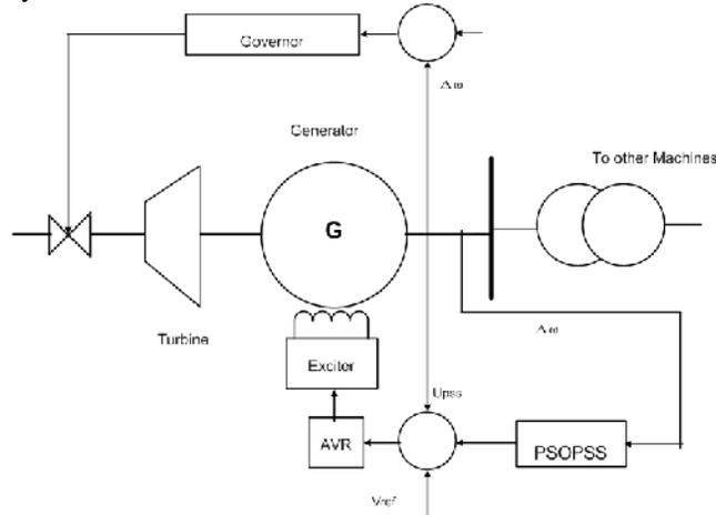
Fig. 2. Single Machine Infinite Bus System.
