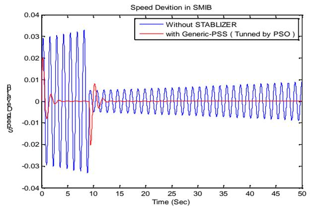
**Fig. 4.** Speed deviation without PSS & with PSO based PSS fault at  $t = 5$  sec ( $\Delta T = 0.05p.u.$ ).
