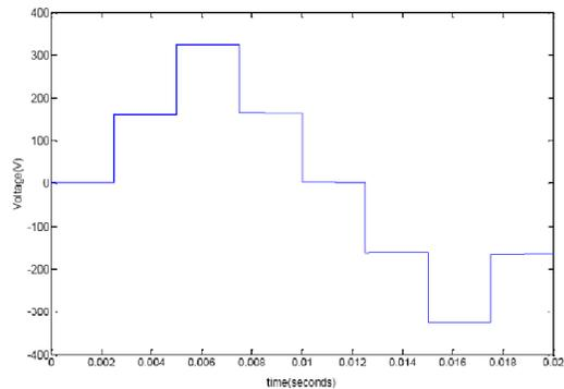
**Fig. 3.** Output voltage of a 5-level multilevel inverter.
