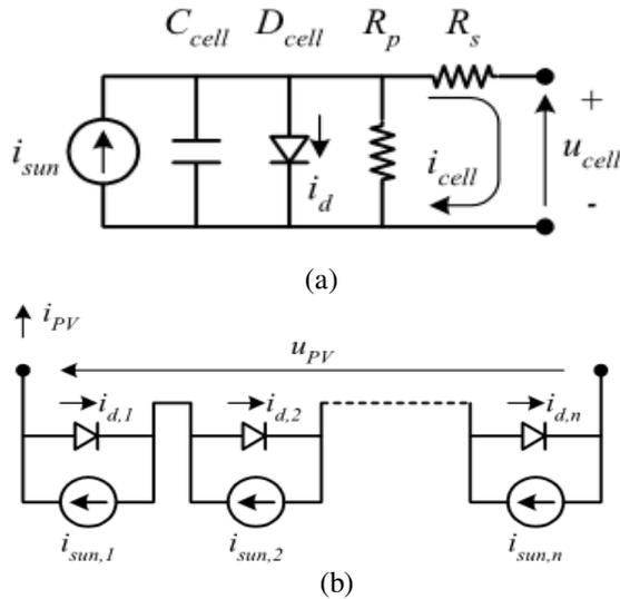
**Fig. 1.** Electrical model of a PV cell (a), and of a PV module made up around n cells (b).
