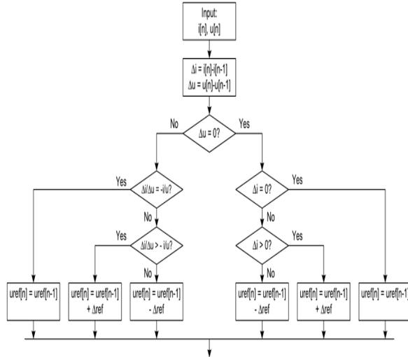
**Fig. 8.** Flow chart of the incremental conductance MPPT algorithm.
