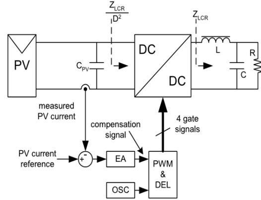
**Fig. 7.** Block diagram of the DC-DC converter with the proposed controllers.
