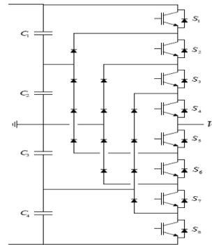
**Fig. 2.** One phase of a diode clamped inverter.
