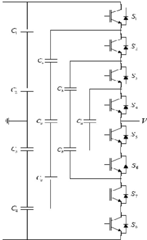
**Fig. 4.** One phase of a 5-level Flying capacitor multilevel inverter.
