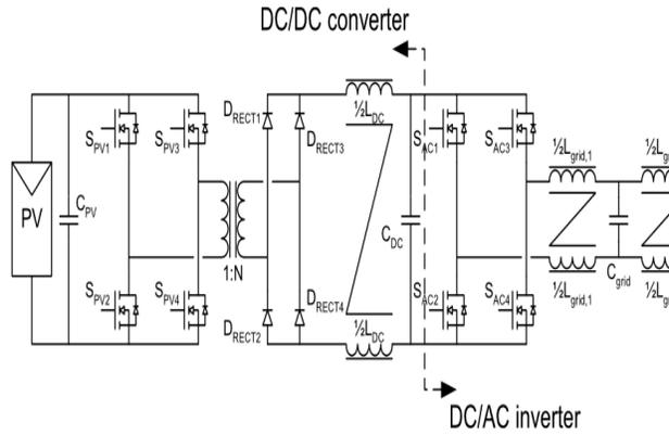
**Fig. 6.** Power circuit of the photovoltaic inverter.
