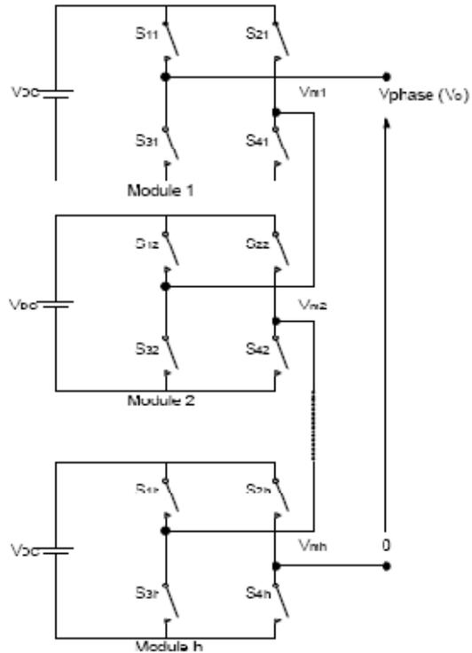
**Fig. 5.** One phase of a cascaded H-bridge multilevel inverter.
