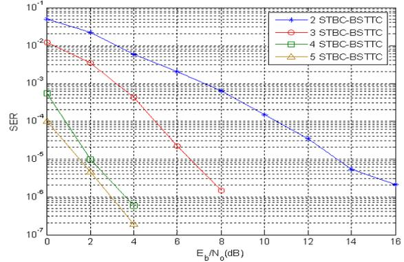
**Fig. 6.** Performance of the system with STBC based B-STTC site diversity for various antennas.
