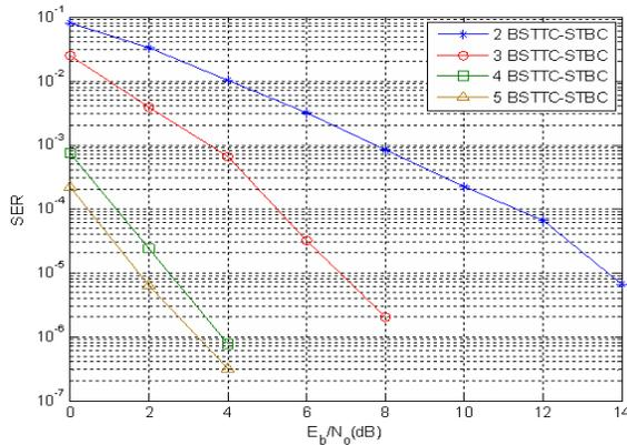
**Fig. 5.** Performance of the system with B-STTC based STBC site diversity for various antennas.
