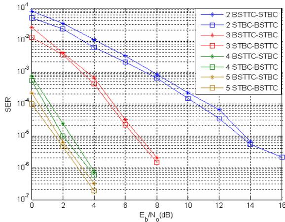
**Fig. 8.** Performance comparison of the system with STBC based STTC and B-STTC based STBC site diversity techniques for various antennas.
