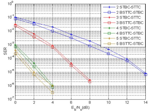
**Fig. 7.** Performance comparison of the system with STBC based STTC and B-STTC based STBC site diversity techniques for various antennas.
