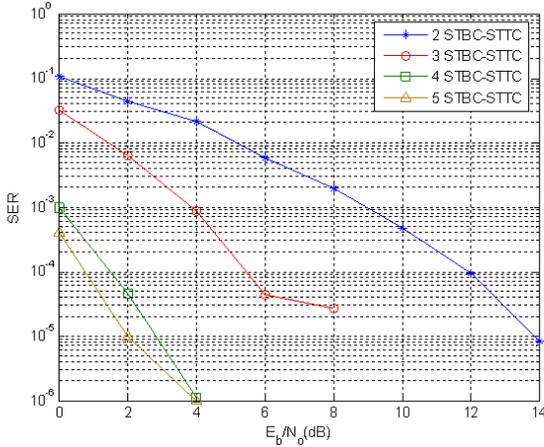
**Fig. 4.** Performance of the system with STBC based STTC site diversity for various antennas.
