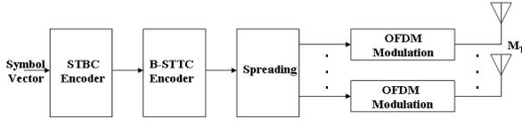
**Fig. 2.** Block diagram of STBC based B-STTC site diversity transmitter for MC-CDMA system.
