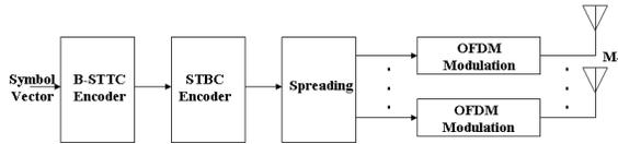
**Fig. 1.** Block diagram of B-STTC based STBC site diversity transmitter for MC-CDMA system.
