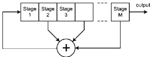
Fig. 4. M-stage Feedback Shift Register.
