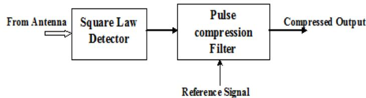
**Fig. 2.** Block Diagram of Non-Coherent Pulse Compression Receiver.
