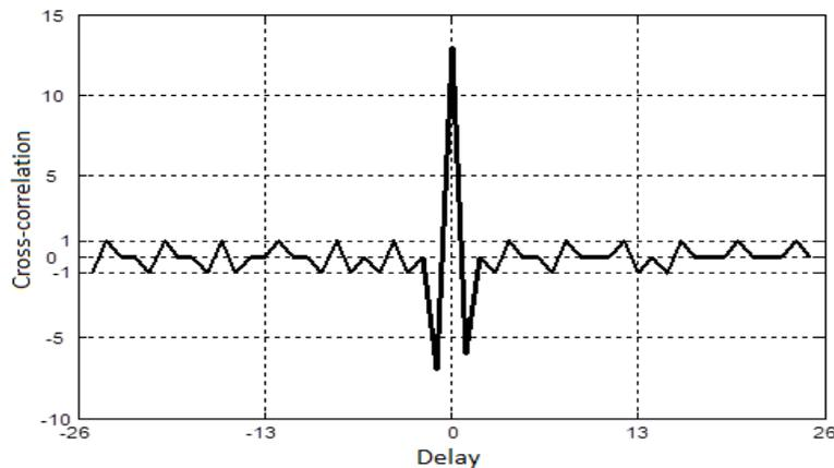
**Fig. 3.** Cross-correlation of the transmitted and reference signals, Barker Manchester code N=26
