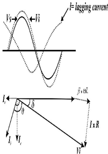
(c) Capacitive mode  $V_s < V_i$ . If  $V_i < V_s$  then I appear to be lagging current this mode. The D-STATCOM will function as a reactor whose inductive reactance is contineously controllable.
