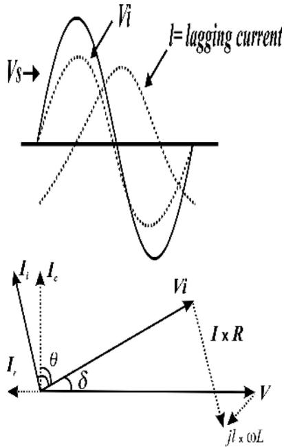
(b) Inductive mode  $V_s > V_i$ , If  $V_s > V_i$  then  $I$  is appear to be leading current since the magnitude of the current can be controlled continuously by adjustint  $V_i$ ,the D-STATCOM will function as a capacitive reactance continuously controllable.
