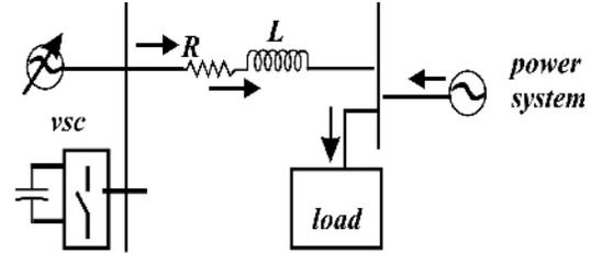
Fig. 2. Basic Building Blocks of the D-STATCOM.
