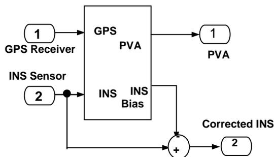
**Fig. 1:** Block diagram of a GPS/INS.
