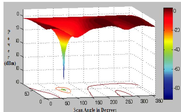
**Fig. 3:** Antenna Array Spatial Processing for Anti-Jamming.
