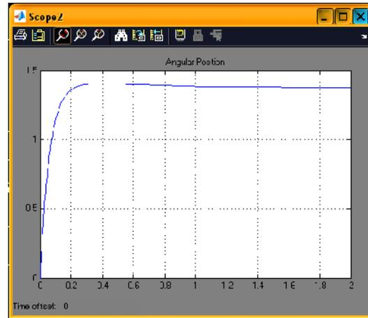
Fig. 14. Angular position for a 0.05pu change in mechanical input with K5 negative with the change in spread of Gaussian membership function.
