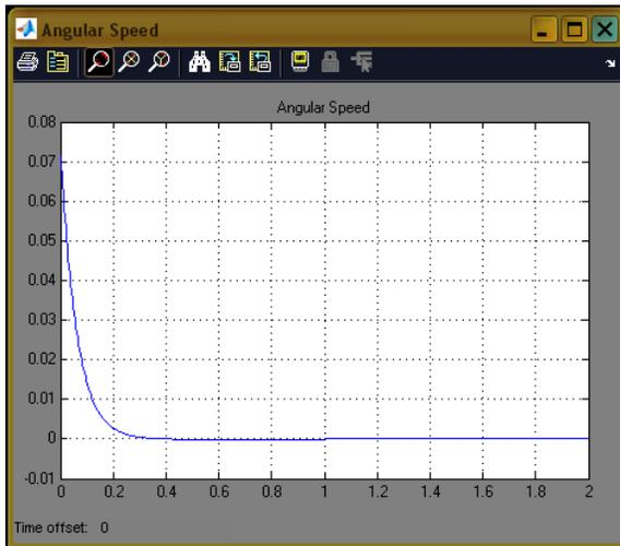
Fig. 13. Angular speed for a 0.05pu change in mechanical input with K5 negative with the change in spread of Gaussian membership function.
