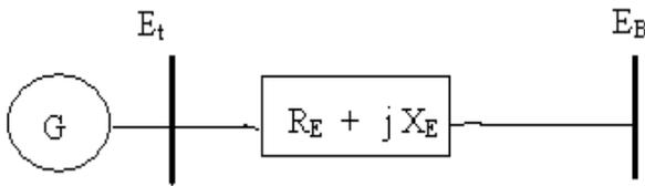
**Fig. 1.** Single machine connected to an infinite bus.
