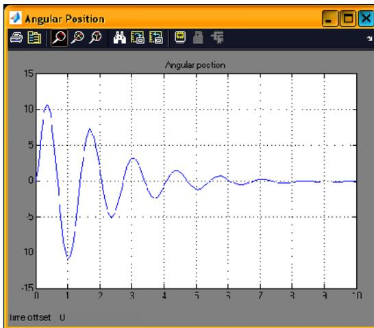
Fig. 9. Angular position for a 0.05pu change in mechanical input with K5 Positive.
