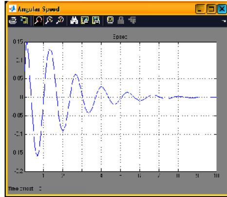
Fig. 10. Angular speed for a 0.05pu change in mechanical input with K5 Positive.
