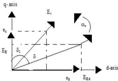
**Fig. 2.** Vector diagram of single machine connected to an infinite bus.
