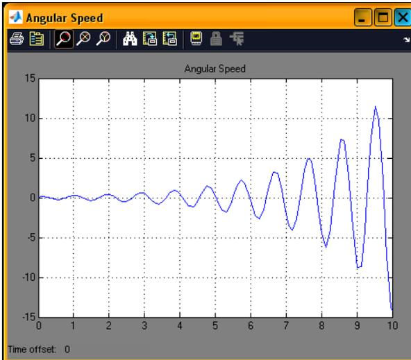
Fig. 12. Angular speed for a 0.05pu change in mechanical input with K5 negative.
