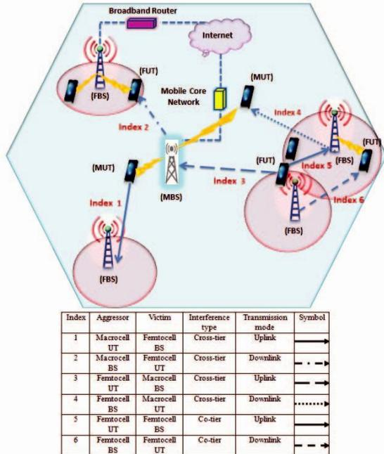
Fig. 1. Interference scenarios in heterogenous networks.
