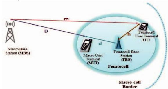
Fig. 2. Example of spectrum sharing between macro and femto cell.
