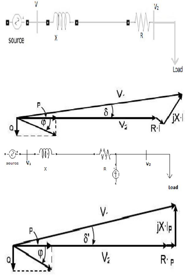
**Fig. 1.** Shunt Compensation.
