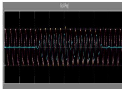
Fig. 3. Waveform of  $I_a$  Prim,  $V_a$  Prim &  $V_a$  Sec in pu with respect to time in Sec.
