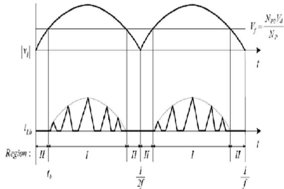
Fig. 5. Operation region of Converter.
