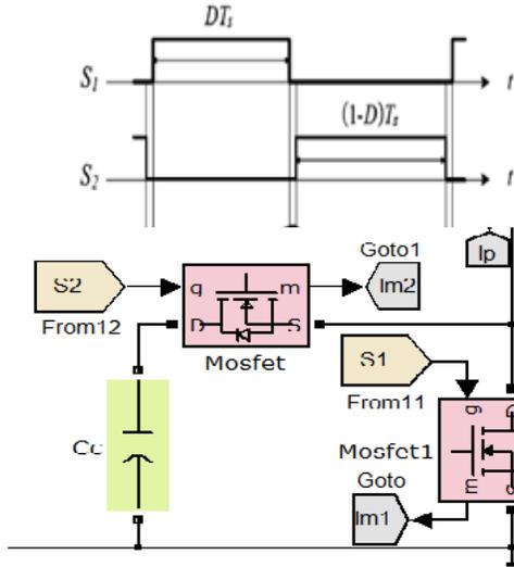
**Fig. 2.** Active clamp circuitry.
