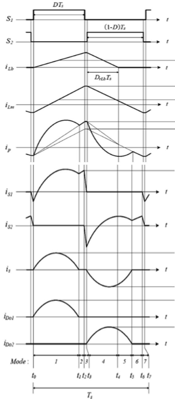
Fig. 6. Key waveforms of the proposed converter.
