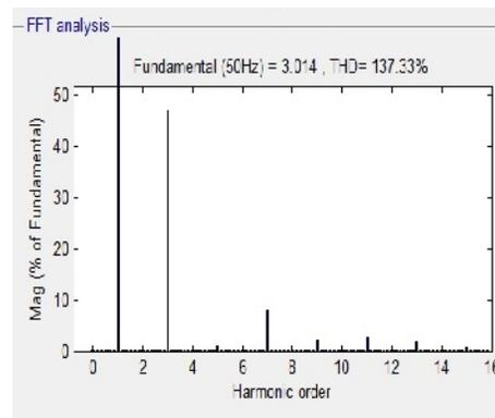
**Fig. 9.** FFT Analysis of Supply Current.
