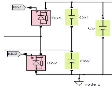
**Fig. 4.** Voltage doubler rectifier schematic.
