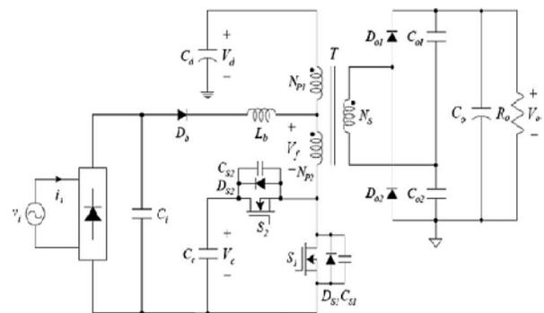
Fig. 1. Circuit diagram of proposed single stage soft switching converter.
