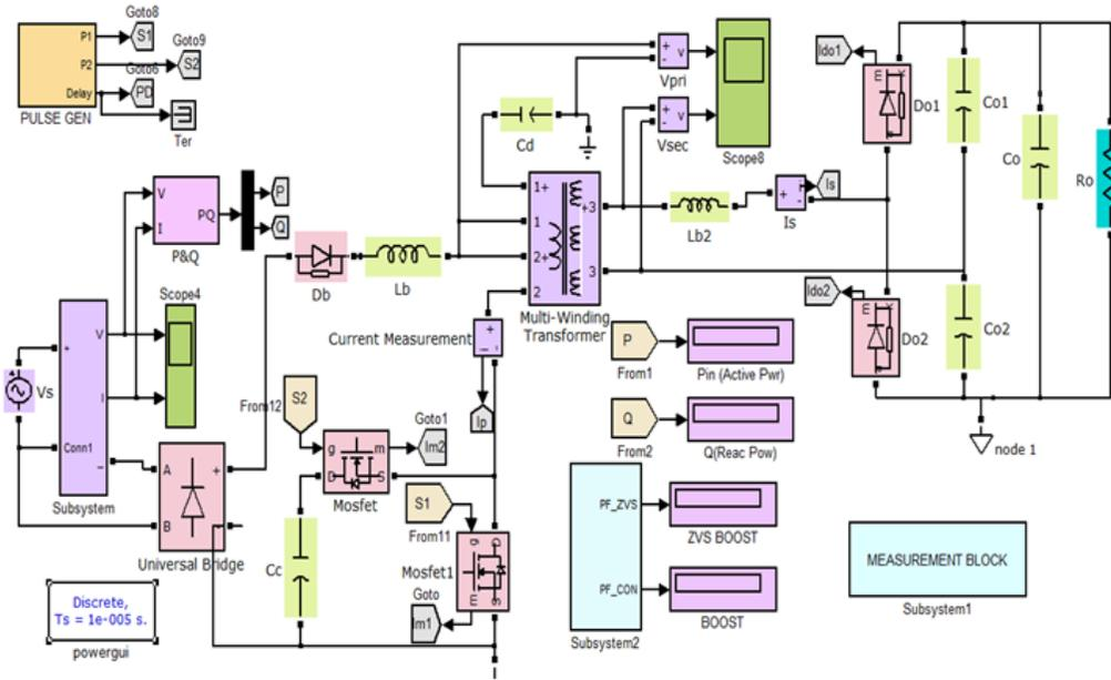
**Fig. 7:** Simulink model Developed for proposed converter.
