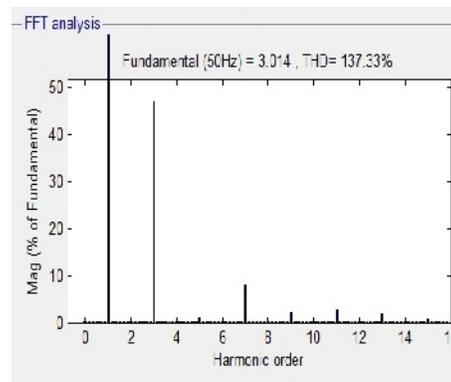
**Fig. 9.** FFT Analysis of Supply Current.
