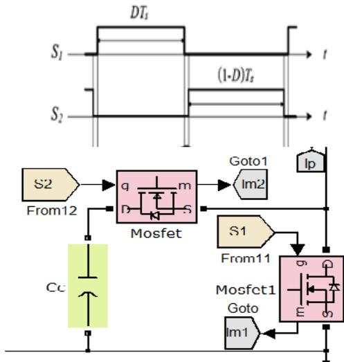
**Fig. 2.** Active clamp circuitry.
