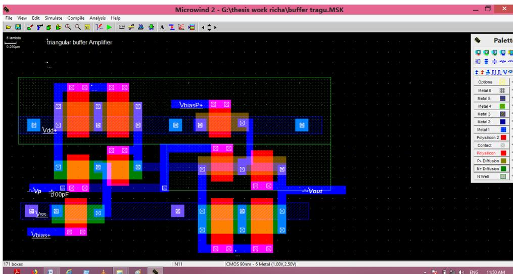
Fig. 2. Layout diagram of the main buffer implemented.
