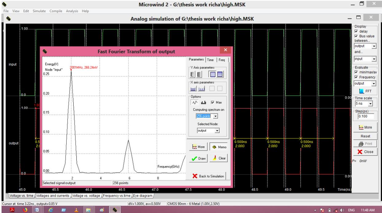
Fig. 5. Input and output waveforms of the voltage with their frequency response.
