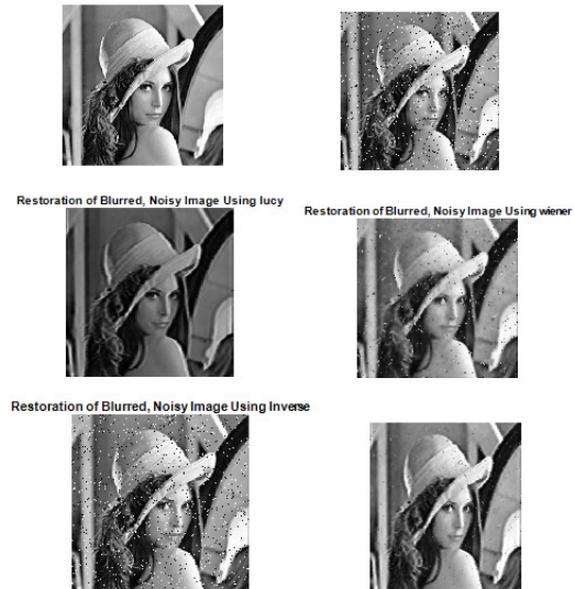
Fig. 1. (a) Original image (b) Blurred and noisy image (c) Image restored by Lucy Richardson (d) Image restored by Wiener filter (e) Image restored by Inverse filter (f) Image restored by wavelet based image fusion.
