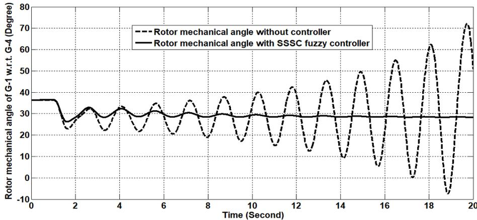
**Fig. 5. Rotor Mechanical angle of G-1 w.r.t. G-4.**
