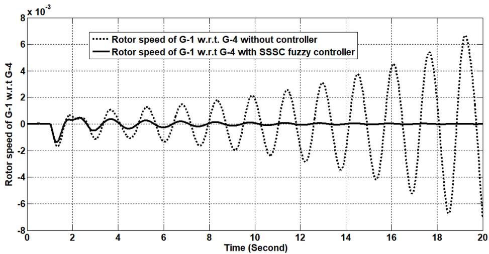
Fig. 8. Rotor speed deviation of G-1 w.r.t. G-4.
