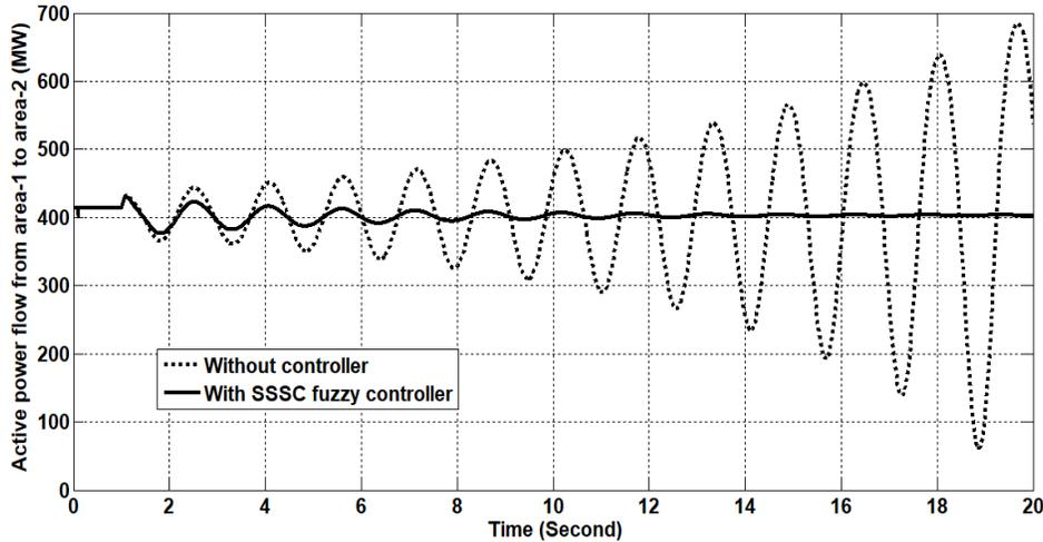
**Fig. 4. Tie-Line Active Power Flow.**
