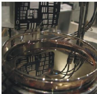
Fig. 3. Five centimeter diameter flat liquid mirror. It is made of an ionic liquid coated with a thin layer of silver. A reflection of a resolution chart is visible in the liquid.
