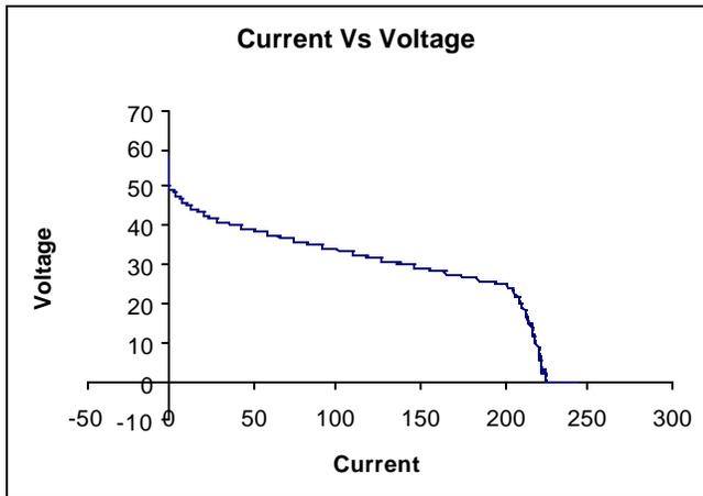
Fig. 11. V-I Curve of the PEM Fuel Cell model
