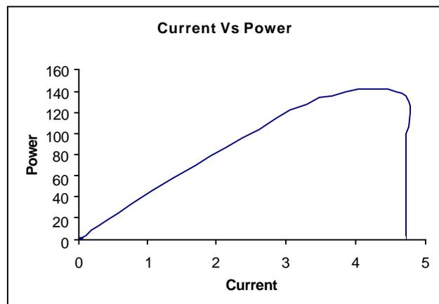
Fig. 9. P-I Curve of the PV model under temperature (25°C)
