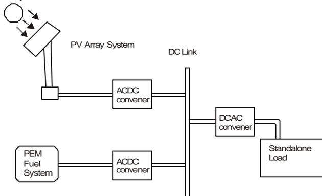
Fig.1 Block Diagram of Photovoltaic-Fuel Cell Hybrid System
