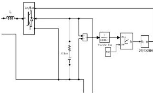
Fig-5 Simulink Model of DC-DC Converter
