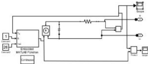
Fig-3 Simulink Model of PV Cell
