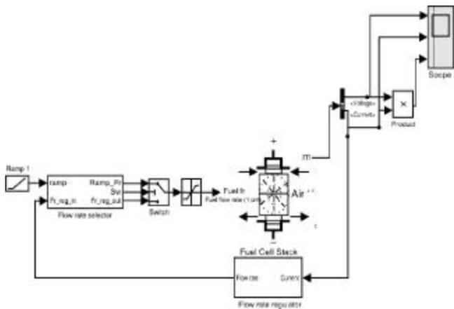
Fig. 4 Simulink Model of PEM Fuel Cell
