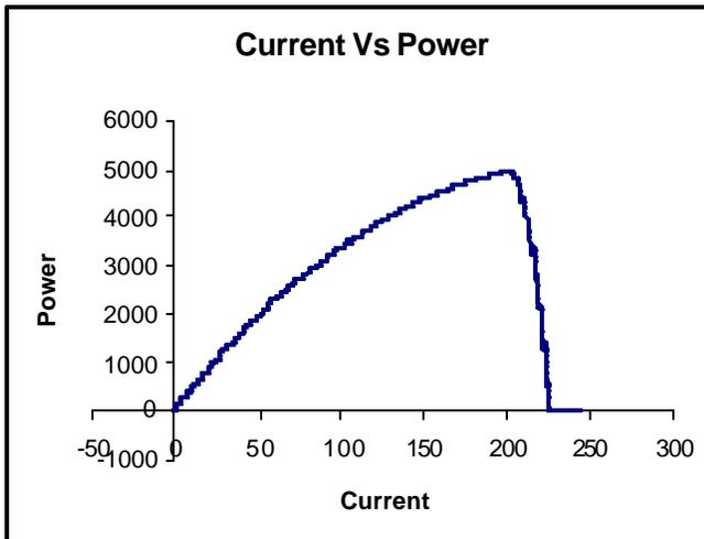
Fig. 12. P-I Curve of the PEM Fuel Cell model
