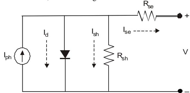
Fig. 2 Electrical model of PV cell
