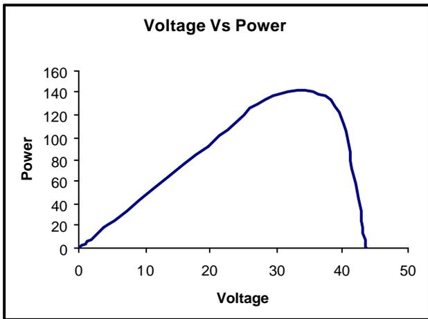
Fig. 7. P-V Curve of the PV model under temperature (25°C)
