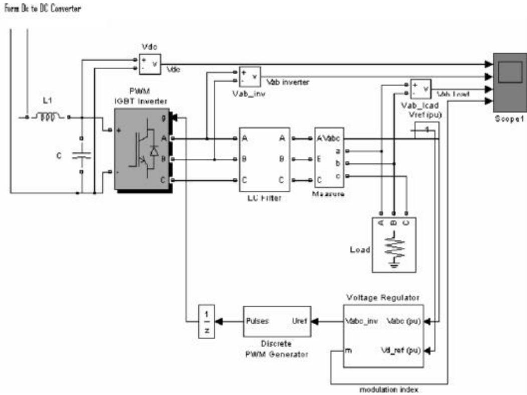
Fig. 6. Simulink Model of the DC-AC Converter
