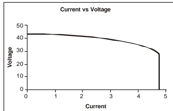
Fig. 8. I-V Curve of the PV model under temperature (25°C)
