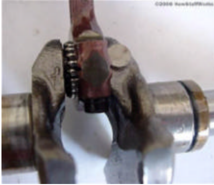
Fig. 4. Functioning of Crank Shaft and bearing. (Courtesy of Howstuffworks.com)
