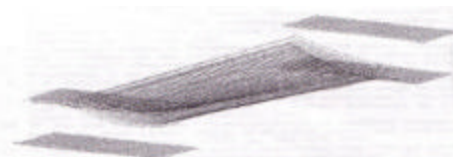
Fig. 5. Point clouds acquired in correspondence with two views of the turbine blade and aligned in a common reference system.
