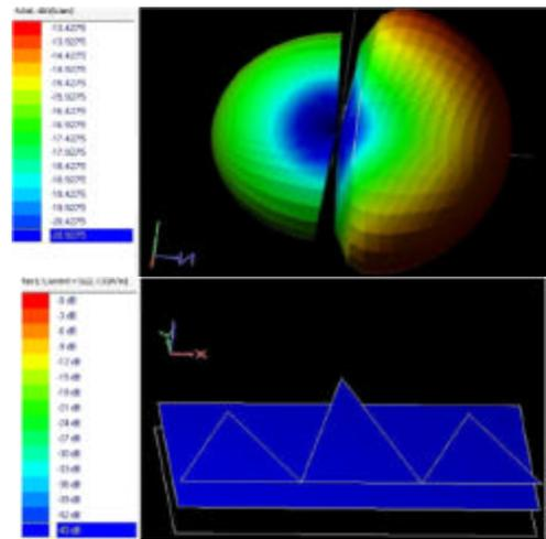
Fig. 10. Radiation pattern & current distribution.
