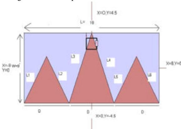
Fig. 7. Triangular shape microstrip antenna.
