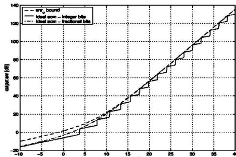
Fig. 4. The output SNR<sub>0</sub> as a function of channel SNR  $\gamma$ , for the SNR<sub>0</sub> bound (dash), the ideal SCM with integer bits (solid) and the ideal SCM with fractional number of bits (dash-dot).  $\gamma = 4$ .
