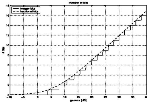
Fig. 3. Number of bits in a digital symbol as a function of channel SNR  $\gamma$ , for an integer no. of bits (solid) and fractional number of bits (dashed).  $\gamma = 4$
