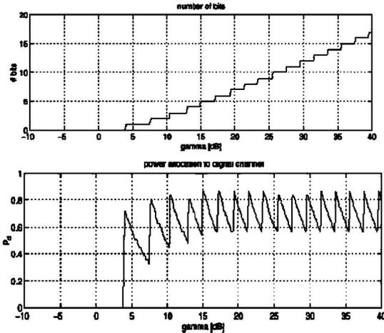
Fig. 6. The number of bits and the optimal power pd as function of  $\gamma$  for the case shown in Fig. 5.  $\beta = 4$
