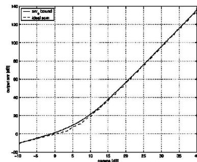
Fig. 5. The output SNR as a function of channel SNR  $\gamma$ , for the ideal case (solid), and the ideal SCM with the integer bits, with power optimization. ( $\beta = 4$ )
