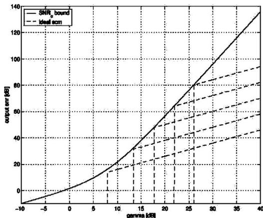
Fig. 7. The output SNR as function of channel SNR  $\gamma$  for the SNR<sub>0</sub> bound (solid), and the ideal SCM with fixed number bits and  $\beta = 4$ . From bottom to top  $b_0 = 2, 6, 8, 10$ .
