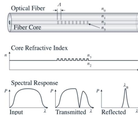
Fig. 1. Bragg grating in optical fiber.
